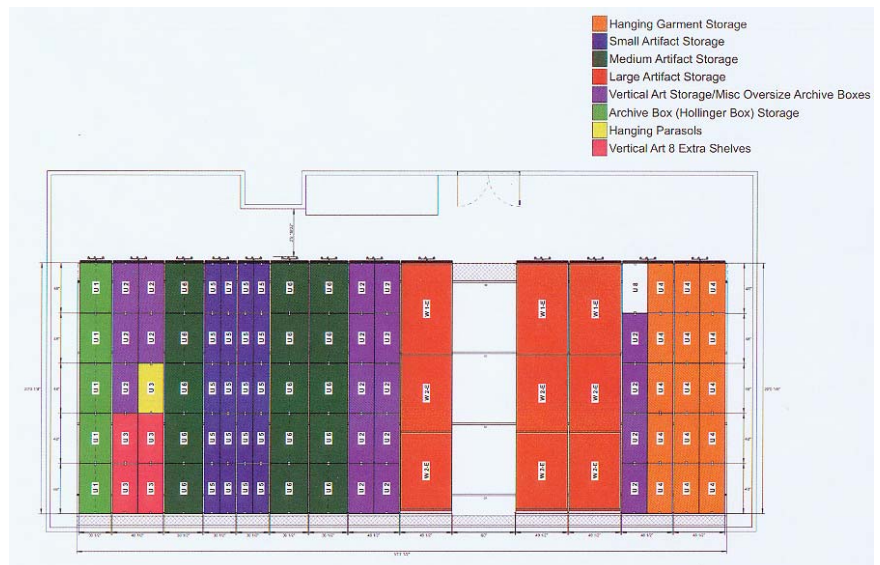
The design, from above, as it will appear with the addition of the four carriages, completing the layout and fully maximize the space within the Storage Room.
